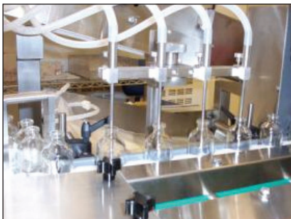
Figure 3. Filling machine with disposable parts
